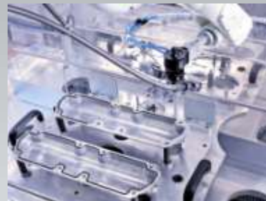
robot applying sealing to cover
