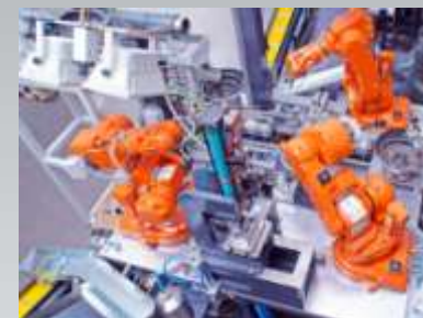
automated single-purpose machine – robotic line
