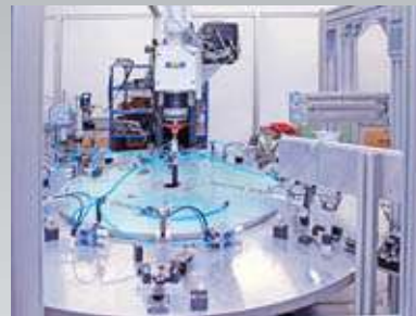
assembly single-purpose machine with rotary table
