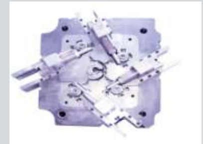
die-casting tool with 4 sliders
